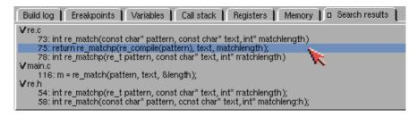
The search results are grouped per file and the corresponding lines containing the searched text are displayed. Double-clicking on one of the lines navigates to the corresponding location in the source code in the editor.
