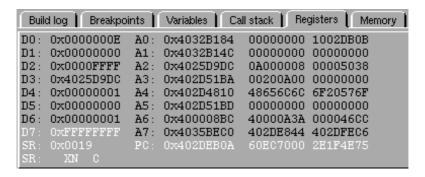
It shows the names and values of the data registers D0-D7 and A0-A7 for addresses, along with the program counter (PC) and status register (SR). By examining these registers, you can monitor changes, diagnose issues, and verify instruction execution.
