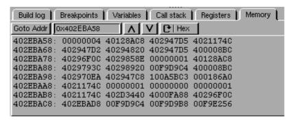
This view helps diagnose issues by providing a detailed look at how data is stored and manipulated. To display a memory area, you can either type the memory address to display into the *Goto Addr* field, or you can double click a variable value in the *Debugger Variable Browser* to display directly to the memory of the variable.
